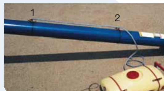
Figure 2: Nozzle placement is important for effective coverage
